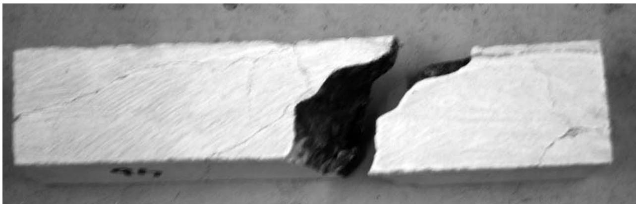
Figure 2. Buixcarró rosa after flexural failure. Note: failure follows clay vein/surface (red).
