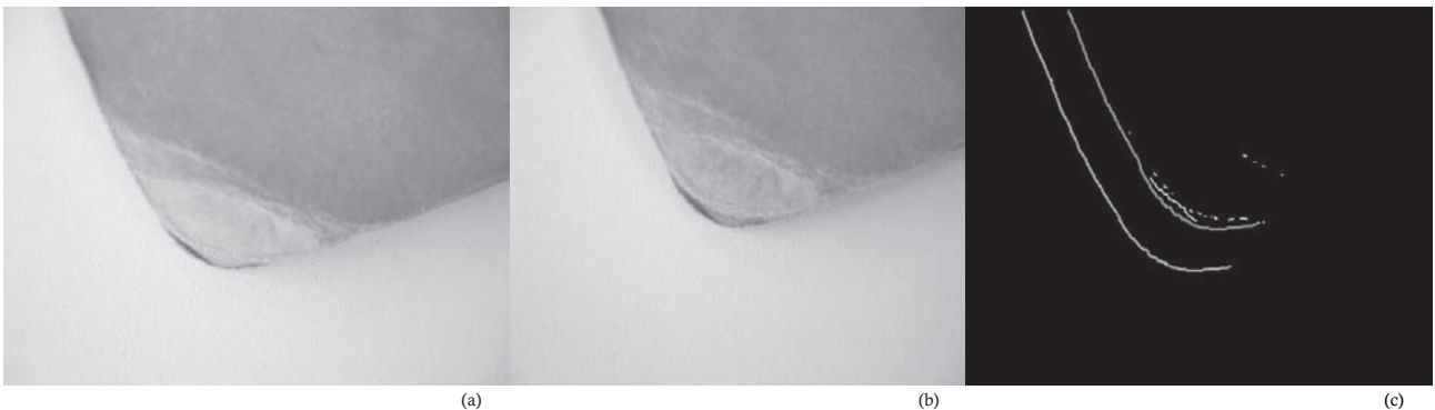
Figure 4. (a) First image in the image sequence; (b) Another image in the image sequence; (c) Borders extracted with Canny (in this case the green and red borders are selected to estimate the object movement after the borders selection process)
