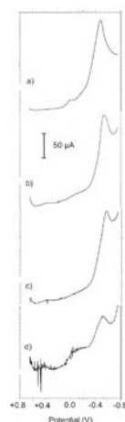
Figure 6. SQWVs of: a) hematite, and samples: b) V1, c) I2, d) O2, immersed into 0.10 M HCl. Potential scan initiated at +650 mV in the negative direction. Potential step increment 4 mV; square wave amplitude 25 mV; frequency 5 Hz
