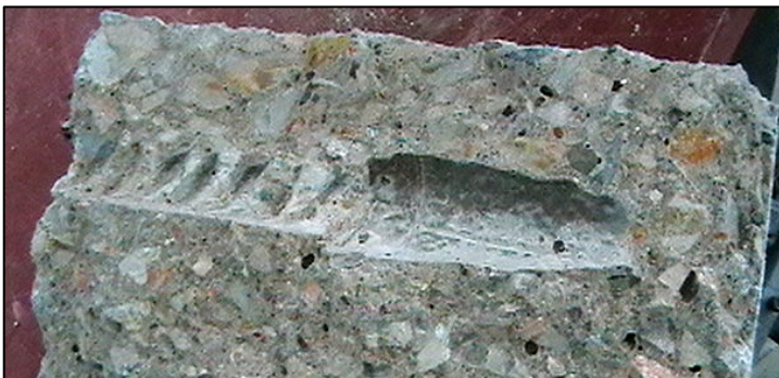
Figure 2.11. Example of splitting failure (detail).
