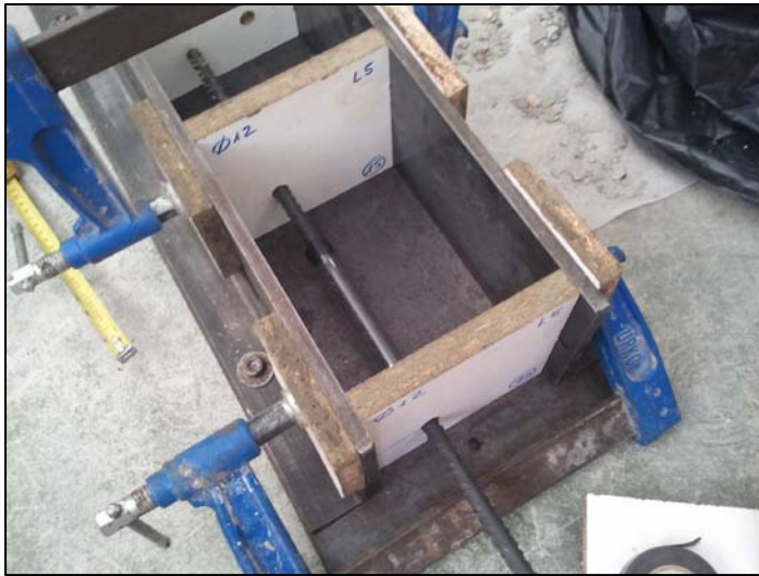
Figure 4.9. Detailed view of a mould for POT specimens.
