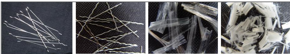
Figure 1.1. Different types of fibers. From left to right: steel (hook-end wire and deformed); polypropylene; poliester.
