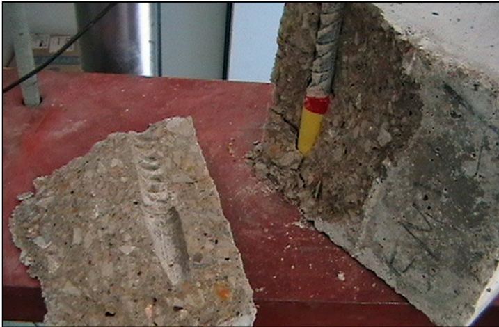
Figure 2.10. Example of splitting failure.
