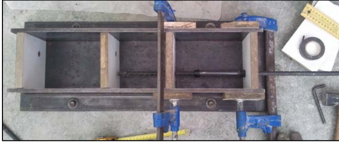
Figure 4.8. A view of a mould for POT specimens.
