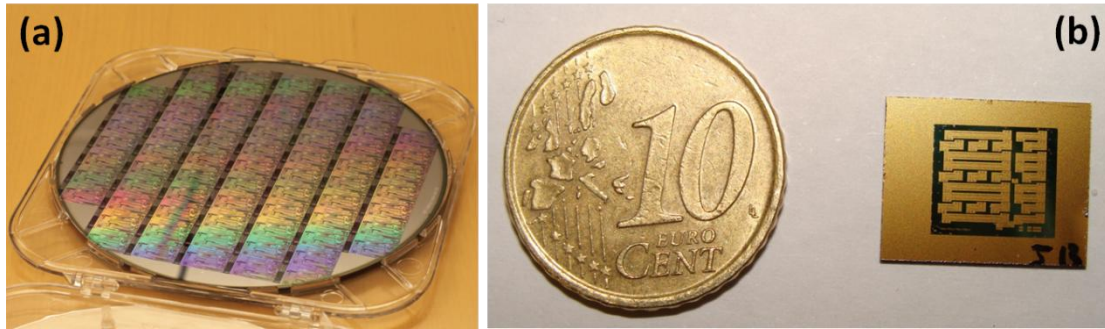
Figure 1-9: (a) Photograph of an 8-in SOI wafer with hundreds of photonic components and circuits and (b) picture of a single silicon chip fabricated in CEA-LETI consisting of 26 electro-optical modulators.
