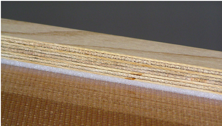
Figure 6.5. Detail of the front bezel showing the EB2 boundary condition with foam.
