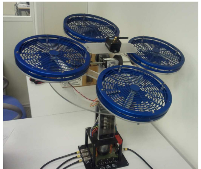
Fig. 5. Quad-rotor system with a wireless Integrated Measurement Unit (IMU).
