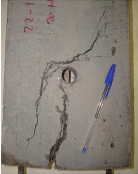
Figure 5.42: Cleavage failure of an element with bar reinforcement and E=150 mm
