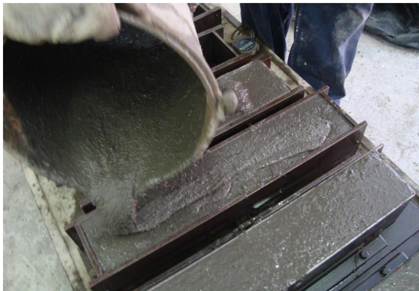
Figure 4.58: Pouring of UHPFRC (Q3-HY) to fill 100 x 100 x 500 mm prisms
