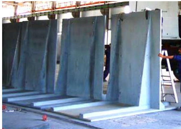
Figure 2.54: Retaining walls made with DURA®
