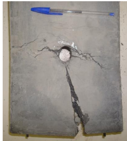
Figure 5.41: Cleavage failure of element with wire reinforcement and E=150 mm
