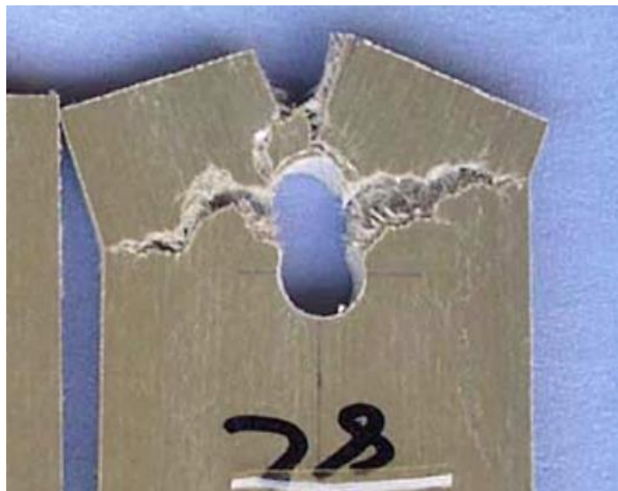
Figure 5.11: Cleavage failure of a pultruded GRP plate
