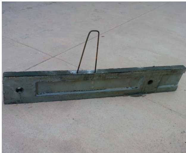
Figure A.6: Tie element 24 h after release (sectional area of 200 x 50 mm at the bolted region)
