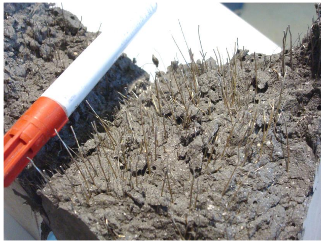
Figure 4.24: Flexural failure section opened, dosage F-6
