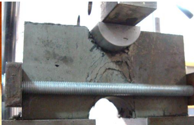
Figure 5.6: Bearing failure of a UHPFRC element
