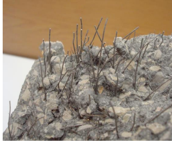
Figure 4.39: Fibers in the section of a tested prism (CA-9)
