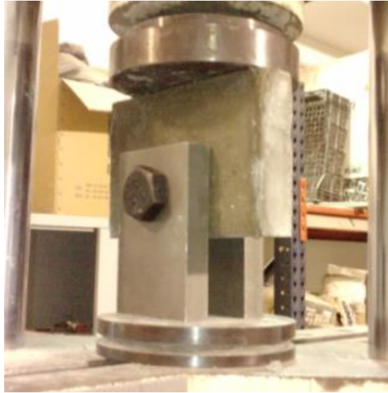
Figure 5.17: Bearing strength test set up
