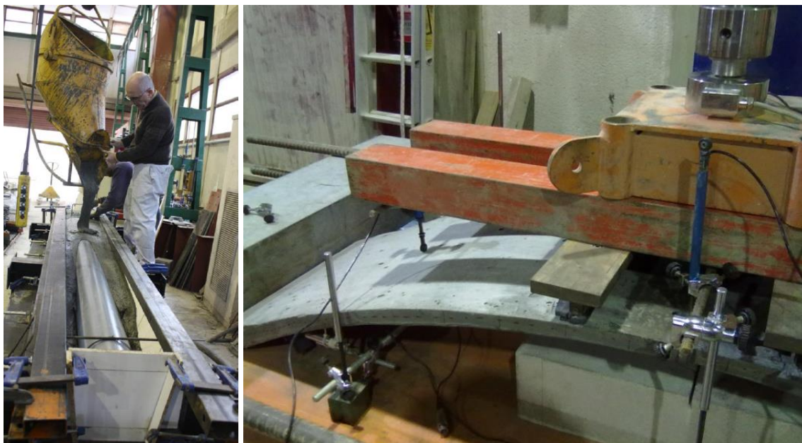
Figure A.9: Three meters length beam being cast
