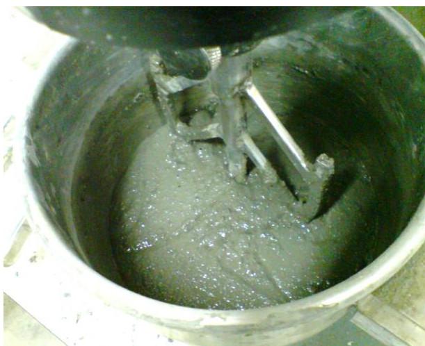
Figure 3.10: Mortar mixer with UHPC
