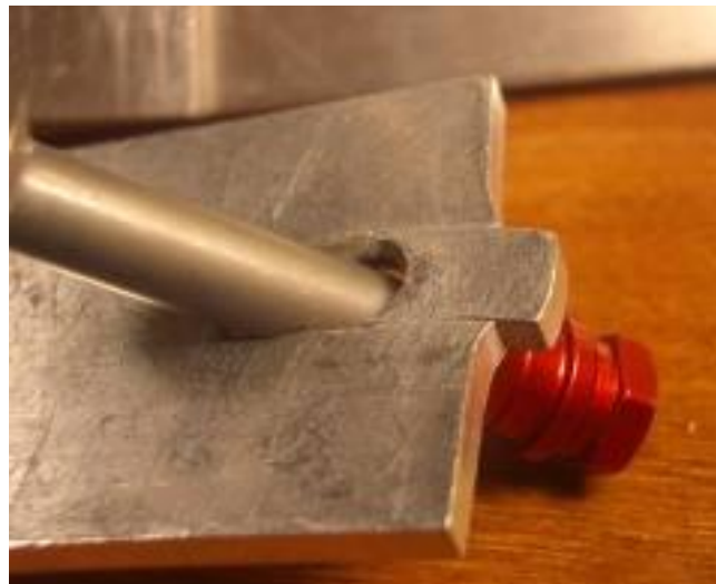
Figure 5.10: Shear out ductile failure
