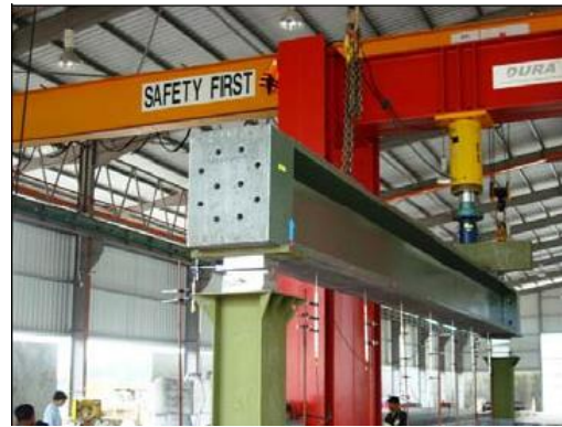
Figure 2.56: Shear test of a rafter beam, where the massive end can be seen
