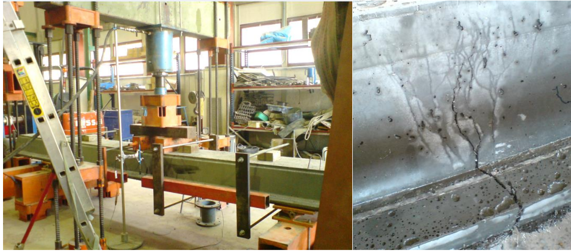
Figure 3.38: Bending test performed to a precast prestressed beam
