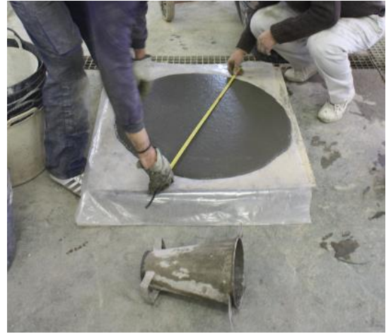
Figure 3.26: Slump flow measurement
