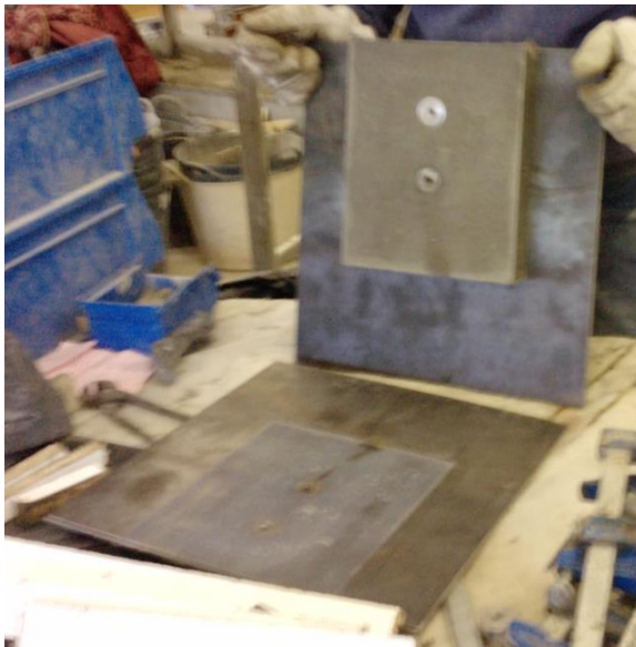
Figure 5.15: Element in the demoulding process. The pouring was made in the vertical position
