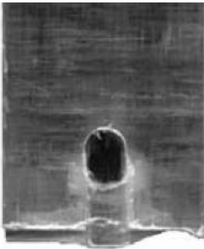
Figure 5.9: Shear out failure of a laminated composite plate [168]
