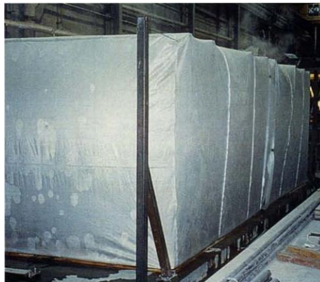
Figure 2.21: Wrapping of an element with polyethylene to apply the steam curing [20]
