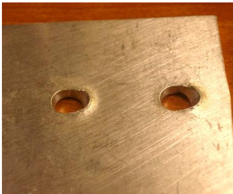
Figure 5.5: Bearing failure in a double bolt steel plate
