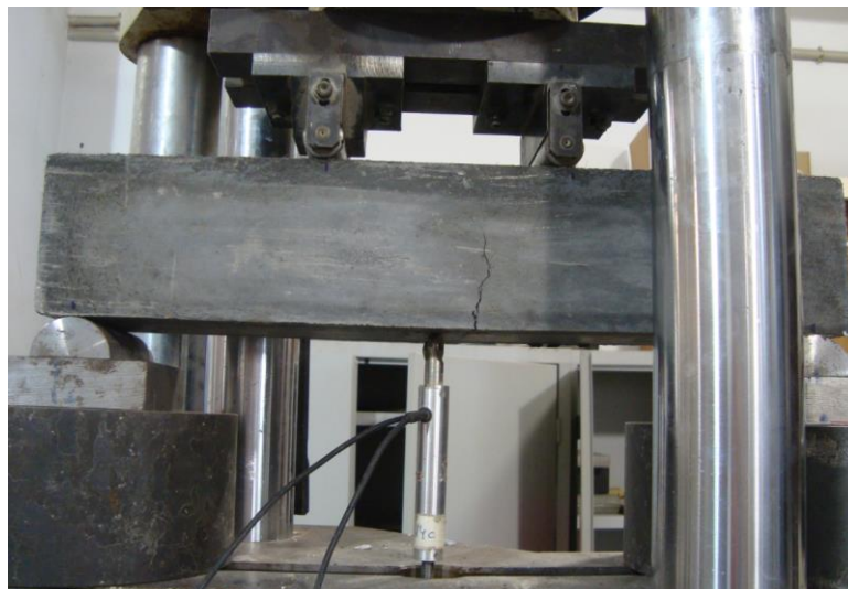
Figure 2.32: Flexural four point bending test
