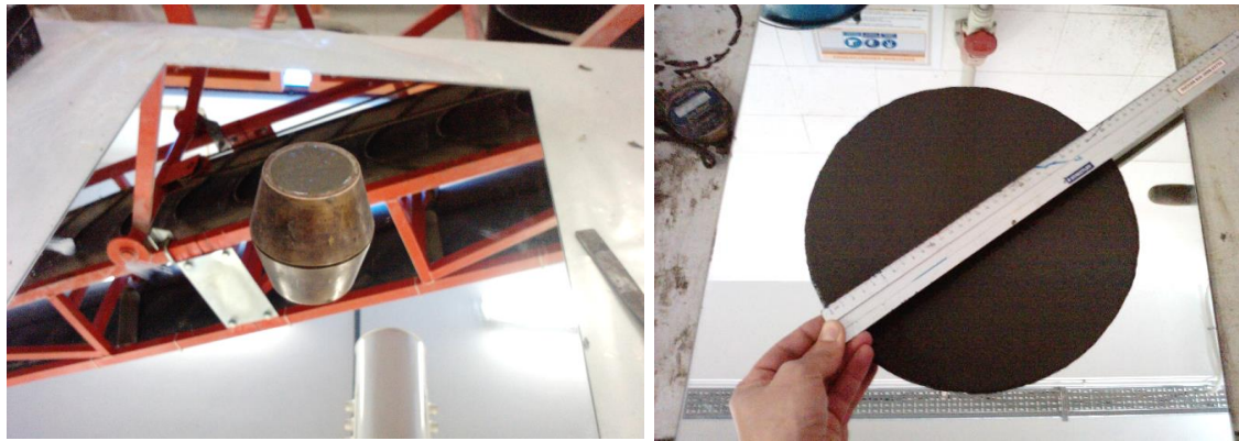
Figure 3.24: Mini-slump cone of one of the mixtures performed in this Ph.D. thesis
