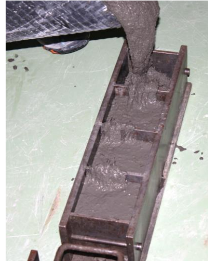
Figure 3.30: Prisms being filled
