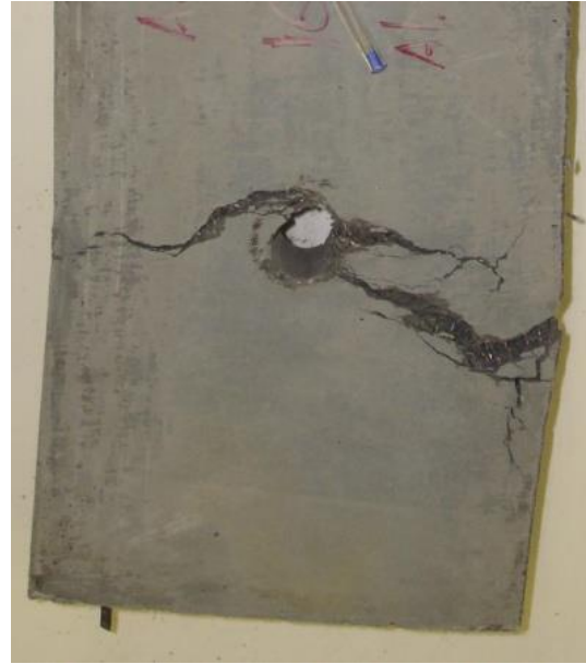
Figure 5.43: Net tension failure mode of element with wire reinforcement and E=150 mm
