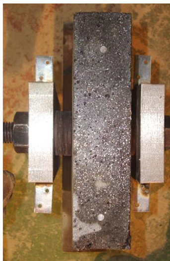
Figure 5.37: piece with the steel shells and bolt, before place it. View from bottom part
