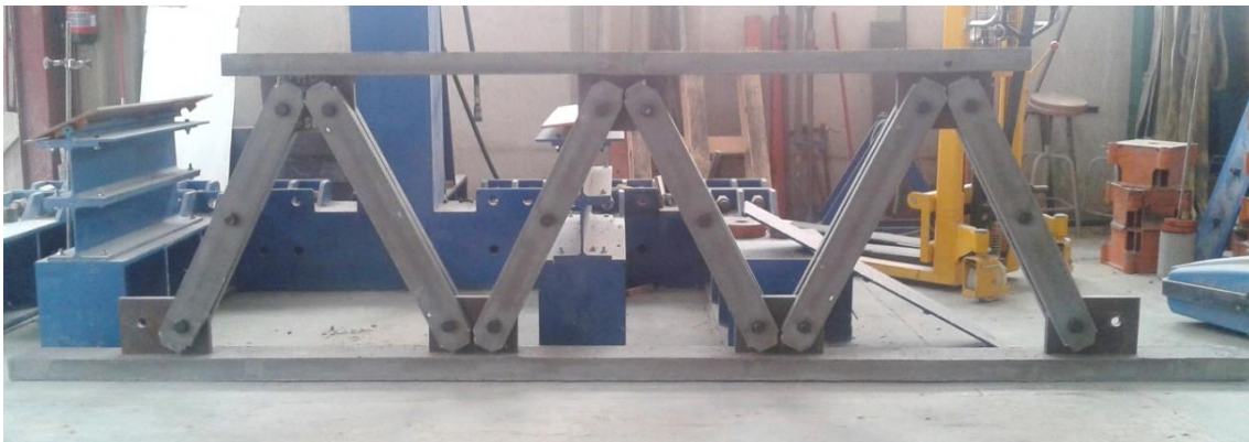
Figure 5.67: Truss element after assembly and before test it
