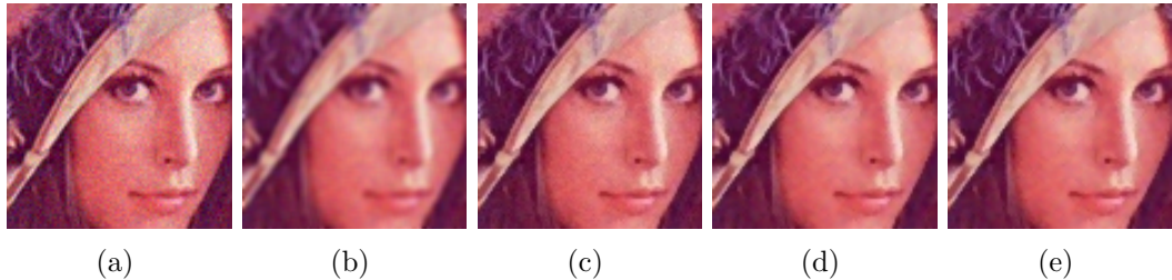
Figure 4: Experimental results: (a) Lenna image contaminated with noise s = 10 and outputs from (b) AMF, (c) FNRM, (d) SSGD C_1 with a = 0.1, b = 0.85 and (e) SSGD C_2 with a = 0.9, b = 1 .
