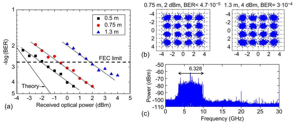
Fig. 4. (a) BER performance of the 19.14 Gb/s single-band system, configuration (A) in Fig. 2, as a function of the received optical power and wireless distance. (b) Constellation diagrams. (c) Electrical spectrum after digitization at the receiver at 2 dBm received optical power and 0.75 m wireless distance.
