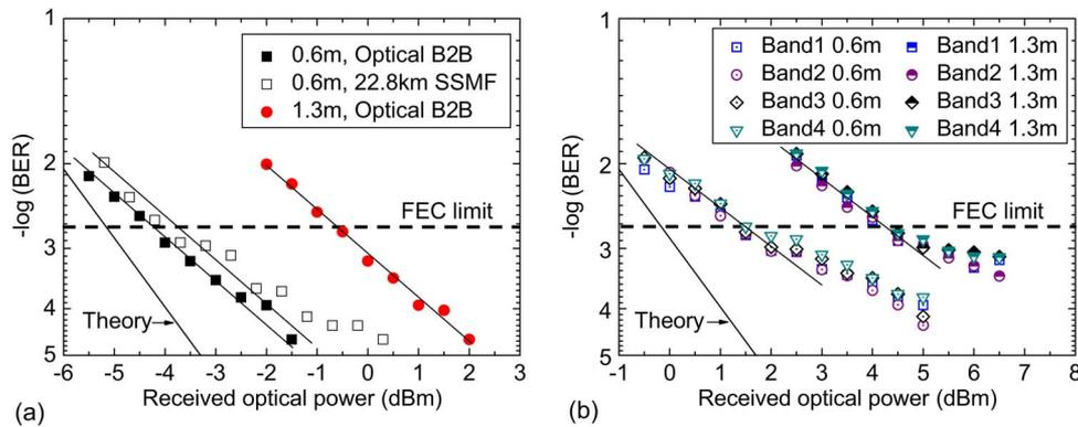
Fig. 6. BER performance of the multiband system, configuration (B) in Fig. 2, as a function of received optical power. (a) 9.57 Gb/s single-band OFDM signal as a function of optical and wireless transmission distance. (b) 9.57 Gb/s/ch four-band OFDM signal as a function of wireless distance for optical B2B.
