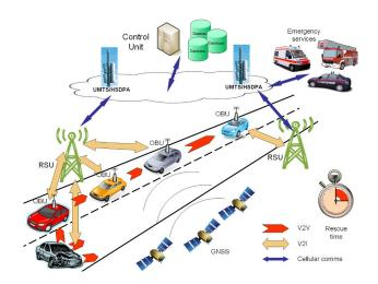
Figure 2. ITS Communication technologies based on the combination of V2V and V2I communications.
