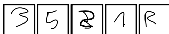
Figure 1.6: Example of handwritten text on a form. The transcription is 3527R. The last field is an error-detecting code that can be computed as the ASCII character at the position 65 plus the numbers in the previous fields ( chr(65 + 3 + 5 + 2 + 7) = 'R' ).
