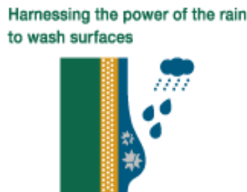
Figure 22. Self-cleaning application with rainwater
