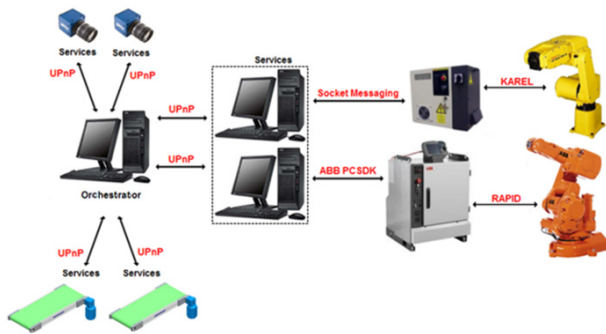
Figure 7. Test bed technological dependences.
