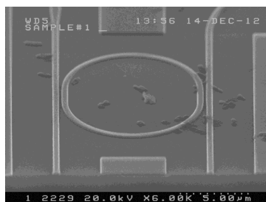
Fig. 4.35: SEM picture of a RR after an assay where PBS and SSC buffers were employed. The deposition of salt particles on the chip surface provokes a variation of the position of the resonances.
