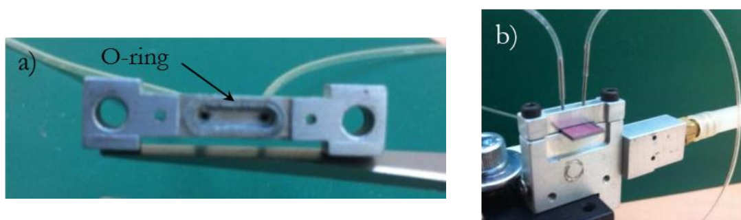
Fig. 3.33: a) Bottom view of the metallic flowcell used to carry out the experiments. Input and output accesses are located on the top of the cavity. A rubber o-ring is placed along the elliptic contour of the cavity in order to achieve a good sealing with the photonic chip. b) Image of the chip holder, where the metallic flowcell is properly placed on top of the photonic chip.
