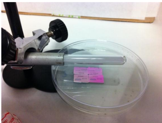
Fig. 4.38: Picture of the UV light exposure during the functionalization of the chip with GOPTS organosilane. Four chips were incubated at the same time to avoid variations in the conditions. The chips were kept in a box to maintain the humidity and the temperature.
