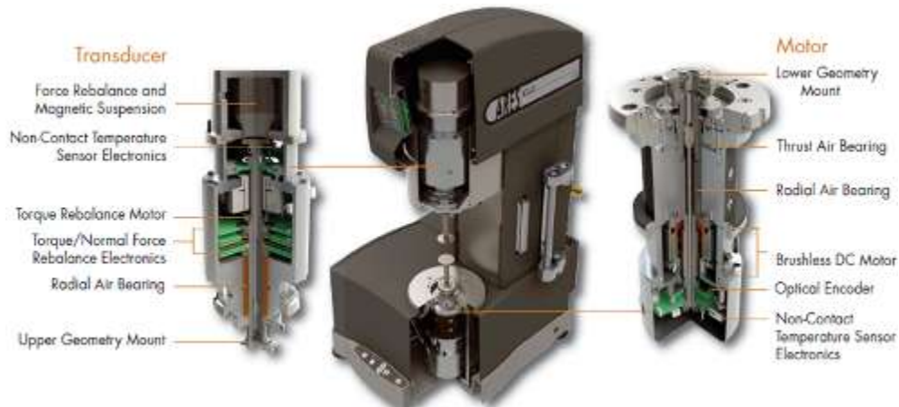
Fig. 6.21. DMA ARES-G2 testing installation, http://www.tainstruments.com/pdf/brochure/AR_Brochure.pdf
