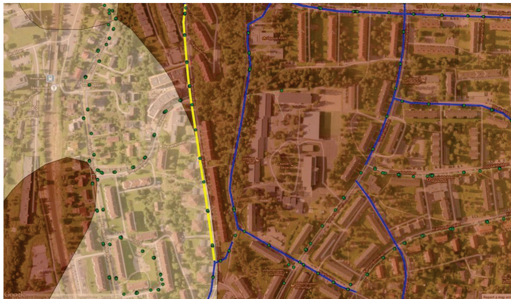
Figure 5.6 Oslo VAV with soil map overlay and maintenance events
