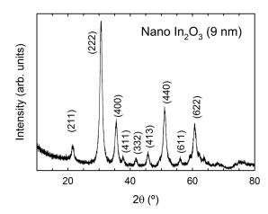
FIG. 1. X-ray diffraction data of nanocrystalline In<sub>2</sub>O<sub>3</sub> obtained at 1 atm.
