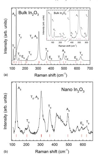
FIG. 2. (a) Unpolarized Raman scattering spectrum of bulk  $In_2O_3$  at room conditions. Inset: Show the spectral regions with smaller intensity Raman modes. (b) Unpolarized Raman scattering spectrum of  $In_2O_3$  nanocrystal. Vertical red lines show the theoretically predicted Raman-mode frequencies at room pressure for bulk  $In_2O_3$  that have been observed experimentally.
