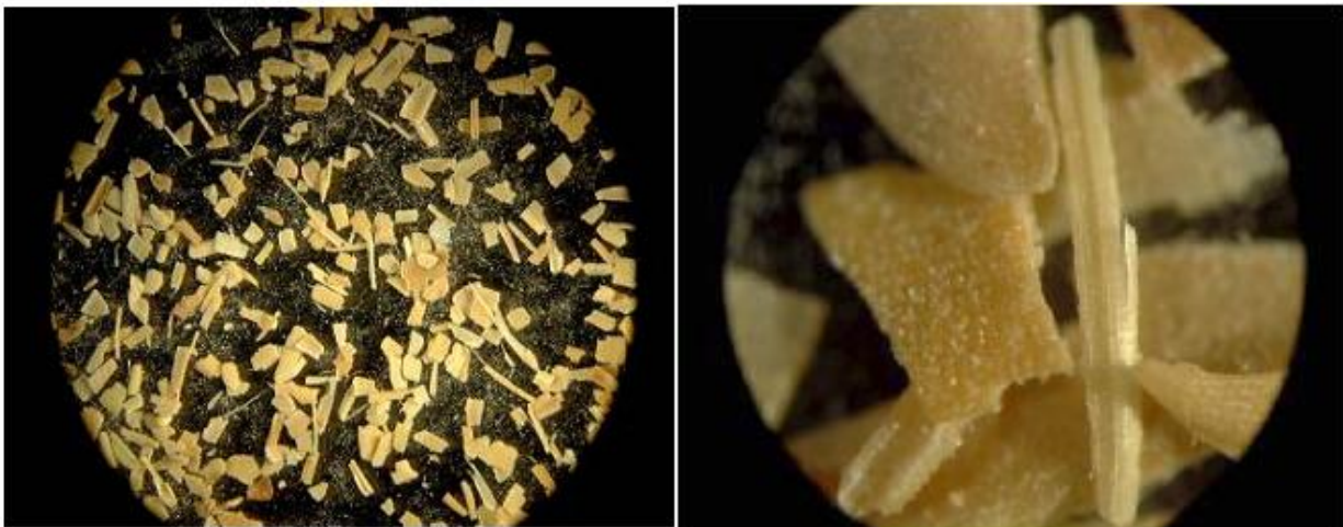
Figure 1. Rice husk particles with granulometry 500 and 1000 \mu\text{m} seen with x10 and x80 magnification lenses.
