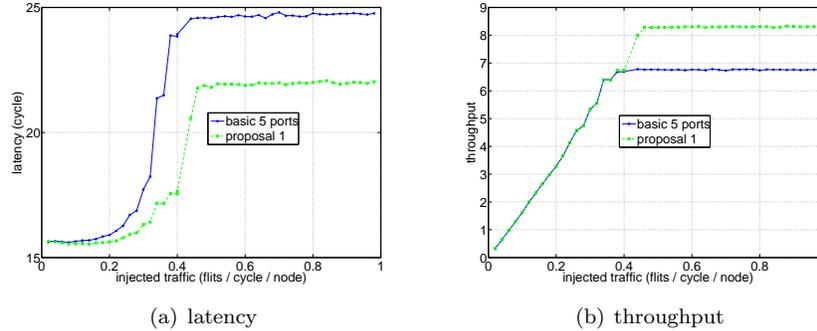
Figure 8: Performance comparison between a basic 5-port switch and proposal 1. All messages are 4-flits long.
