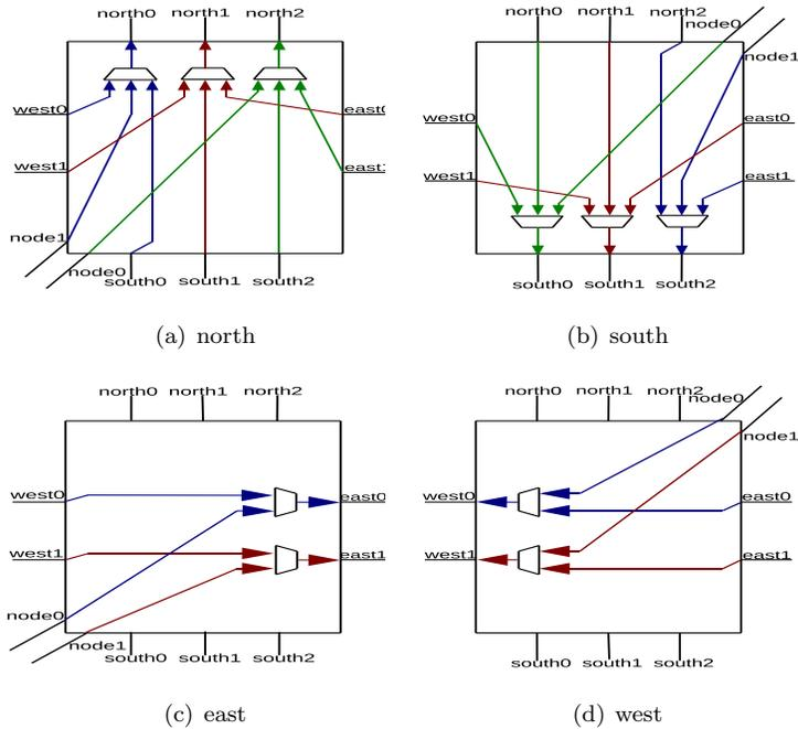
Figure 4: Ad-hoc switch connectivity proposal 2.
