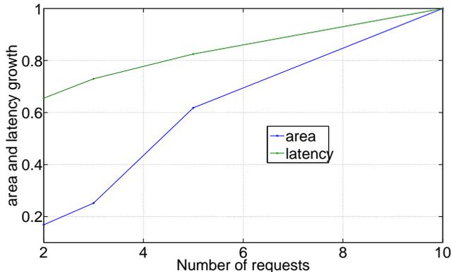
Figure 2: Area and latency of the arbiter growth with respect to the number of requests.
