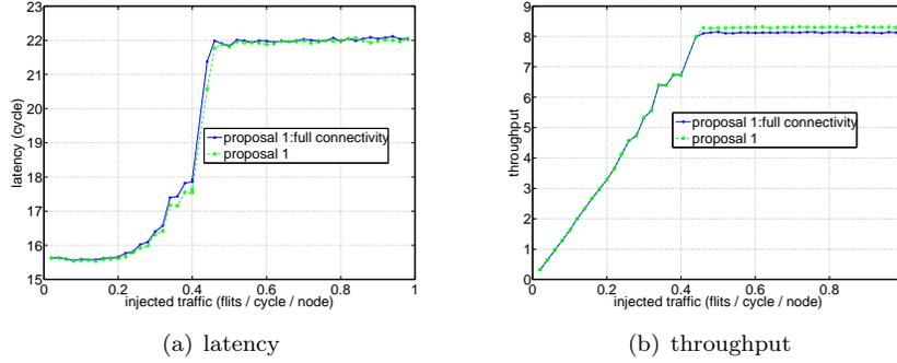
Figure 7: Latency and throughput for proposal 1. Full connectivity for proposal 1 is also considered.
