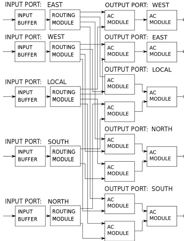
Figure 6: Schematic of the new switch architecture proposed.
