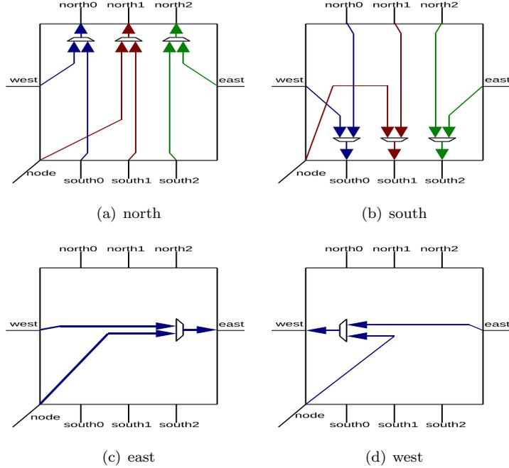
Figure 3: Ad-hoc switch connectivity proposal 1.
