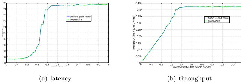
Figure 12: Performance comparison between a basic 5-port switch and proposal 3. All messages are 4-flits long.
