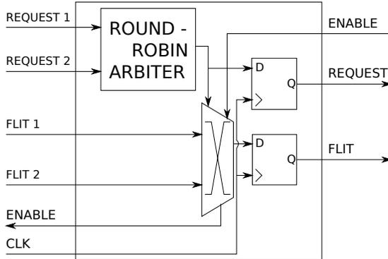
Figure 5: Schematic of the AC module used to implement our new switch architecture.
