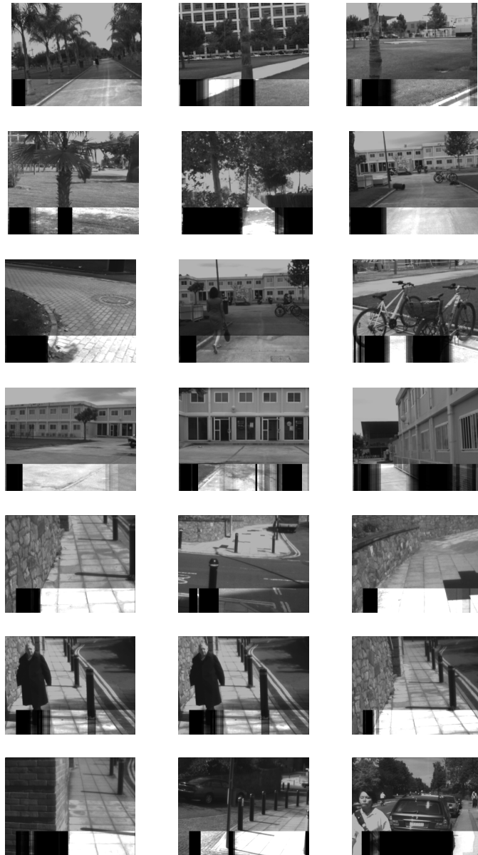
Fig. 6. Processed testing images set. Brighter areas show detected free-paths. Darker areas indicate that they have smaller certainties to be an obstacle-free path.
