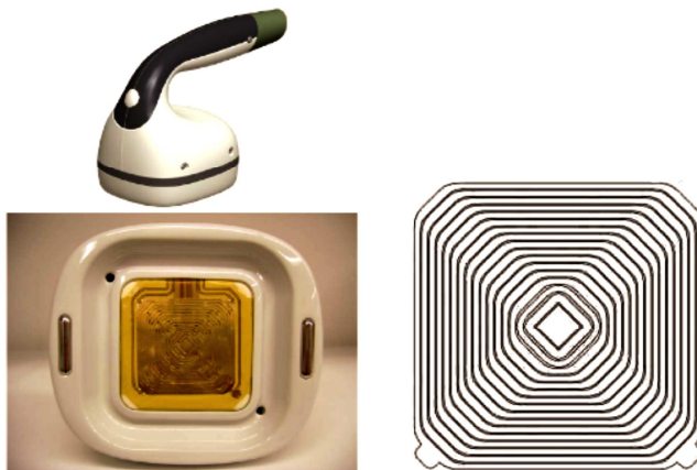
Figure 1.13. RF monopolar applicator which consists of a multidimensional series of tightly spaced concentric rings. Detail of the concentric rings geometry (right).
