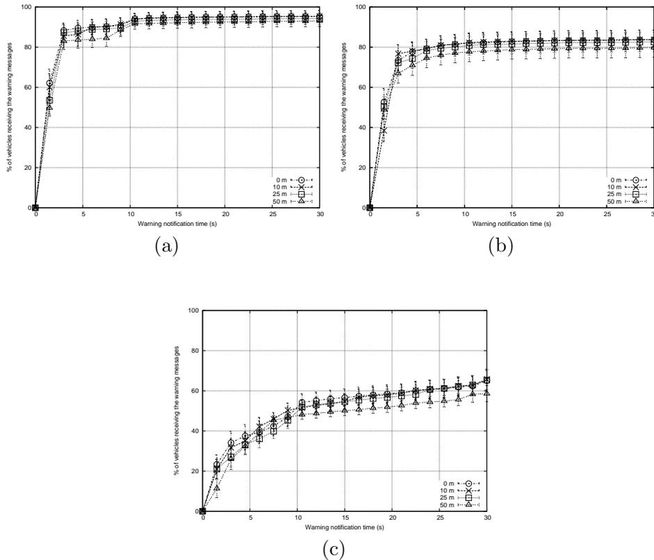
Figure 9: Average notification time and percentage of vehicles informed obtained when simulating 200 vehicles under different levels of GPS inaccuracy and varying the simulation scenario: (a) New York, (b) Madrid, and (c) Rome.
