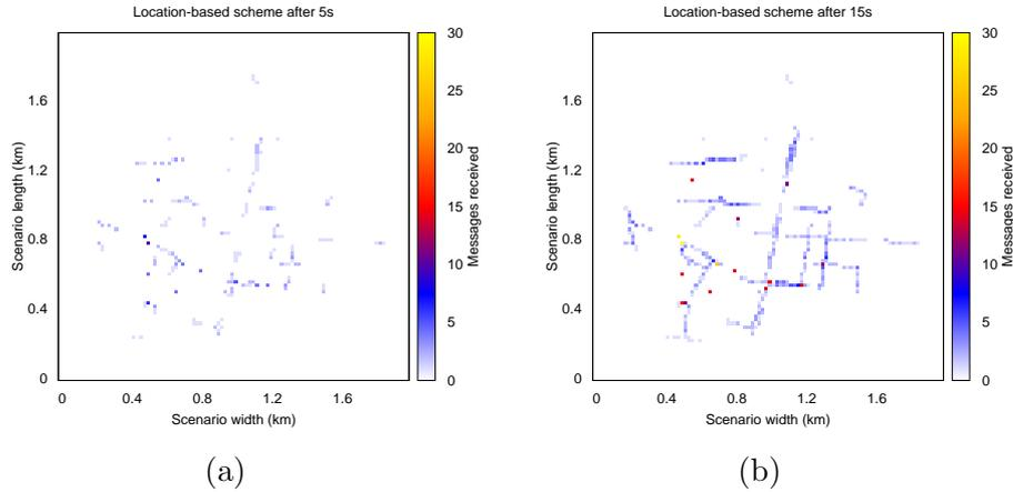
Figure 11: Evolution of the warning message dissemination process in the Madrid scenario simulating 100 vehicles and using a location-based scheme after (a) 5 seconds and (b) 15 seconds.
