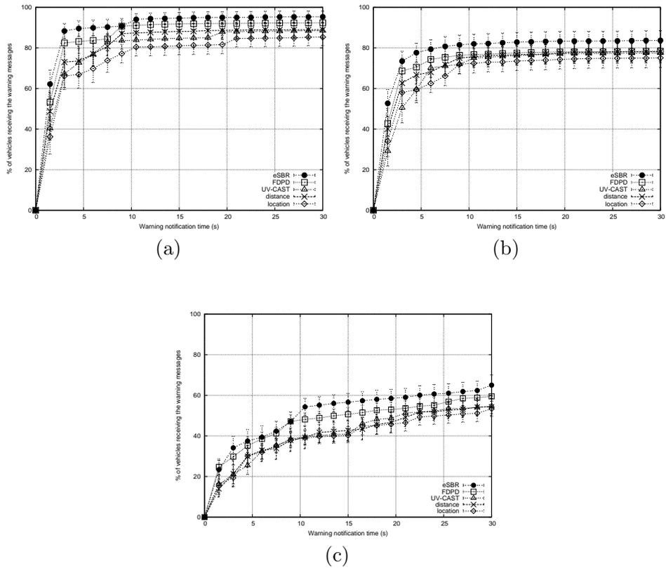
Figure 5: Average notification time and percentage of vehicles informed obtained when simulating 200 vehicles and varying the simulation scenario: (a) New York, (b) Madrid, and (c) Rome.
