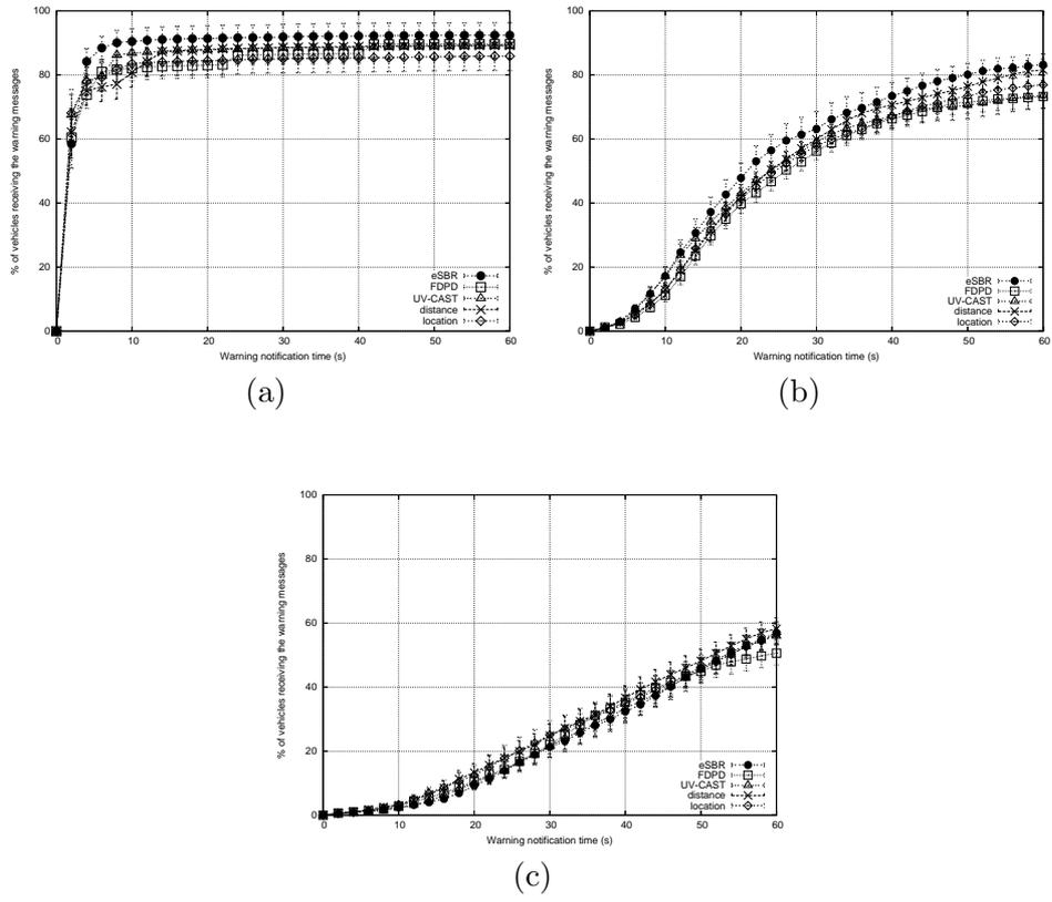
Figure 10: Average notification time and percentage of vehicles informed obtained when simulating 400 vehicles in the Madrid scenario under different levels of background traffic: (a) only warning message dissemination, (b) additional 1 MB/s broadcast by each vehicle, and (c) additional 2 MB/s broadcast by each vehicle.
