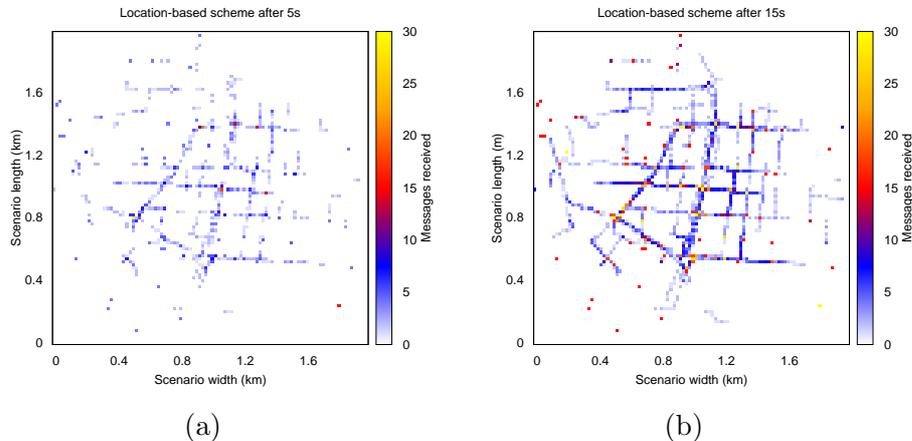
Figure 13: Evolution of the warning message dissemination process in the Madrid scenario simulating 400 vehicles and using a location-based scheme after (a) 5 seconds and (b) 15 seconds.
