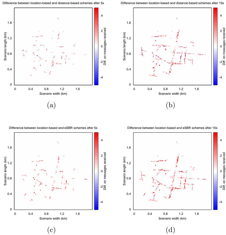
Figure 12: Differences in number of messages with respect to the location-based scheme simulating 100 vehicles in the Madrid scenario; using a distance-based scheme after (a) 5 seconds and (b) 15 seconds, and our proposed eSBR after (c) 5 seconds and (d) 15 seconds.
