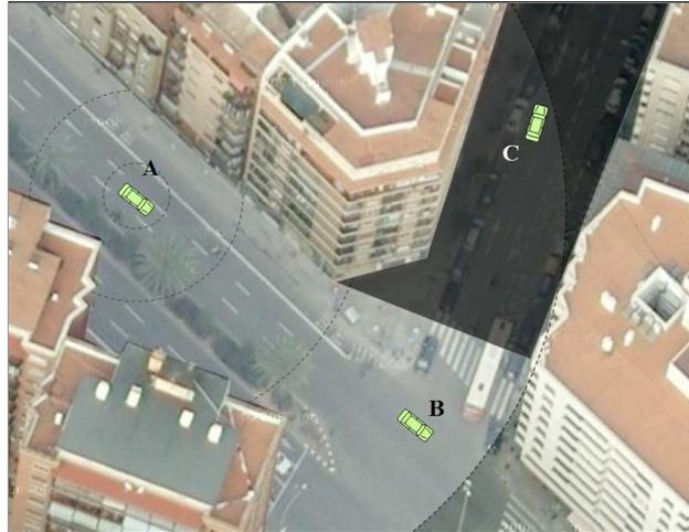
Figure 1: Example of wireless signal propagation in an urban scenario extracted from Google Maps. The lightest area represents the transmission range in a obstacle free environment, and the darkest area indicates the zone where the signal would not be propagated due to blocking by the nearby building.
