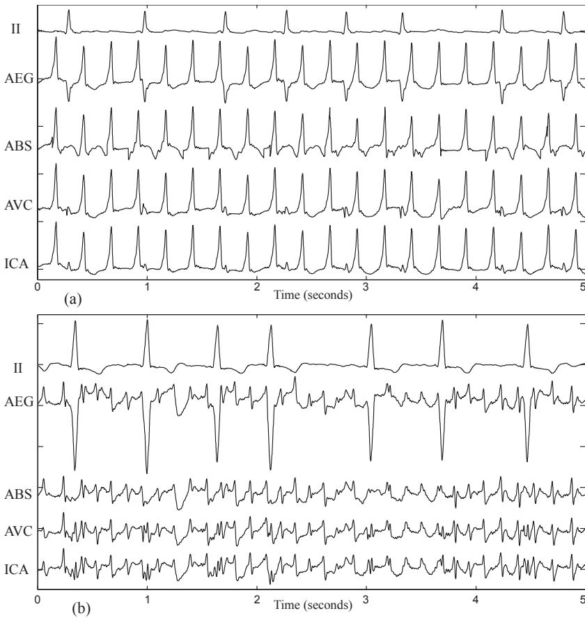
Figure 6. (a) From top to bottom, Lead II of an organized AF ECG shown for reference, the corresponding epicardial atrial electrogram (AEG), result of ventricular reduction with average beat subtraction (ABS), adaptive ventricular cancellation (AVC) and independent component analysis (ICA). (b) This panel plots the same information as panel (a) for a disorganized AF ECG. Note how ABS does not distort the resulting signal in this latter case [31].
