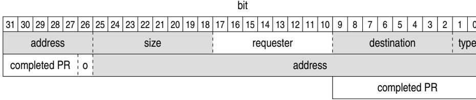
Figure 4: Priority request format. *Type* is the packet type (transient request, response, or priority request). *Size* is the size of the payload (*address*, *o*, and *completed PR* fields). *O* indicates the requested operation (load or store). *Completed PR* is an identifier necessary to inform about the completion of priority requests (for greater detail see [27, 10])
