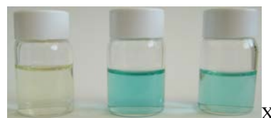
Fig. 2 Colour changes observed for probe 2 ( 1.0 \times 10^{-5} mol dm -3 ) in acetonitrile upon addition of 100 equivalents of DCNP (middle) and 100 equivalents of DFP (right)
