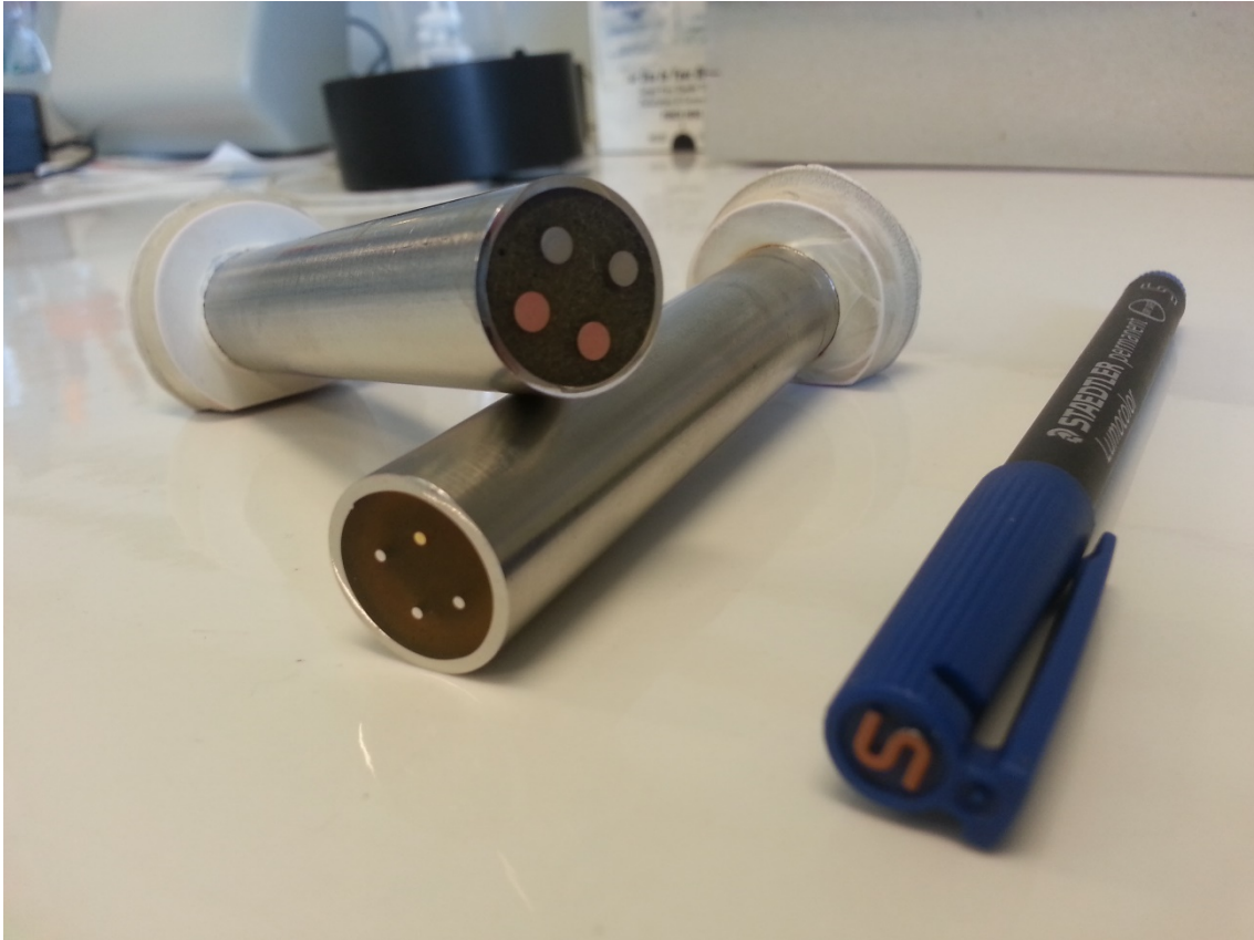
Figure 1.- Example of the designed electrode arrays.
