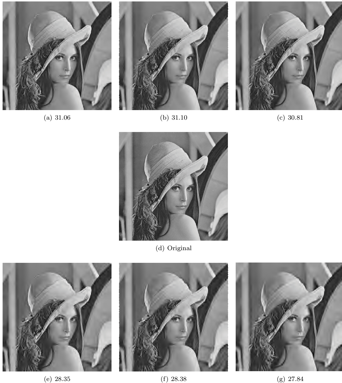
Fig. 11 Lena compressed at 0.125 bpp (a) LTW_RCi_2%, (b) SPIHT, (c) JPEG2000 and Lena compressed at 0.0625 bpp (e) LTW_RCi_2%, (f) SPIHT, (g) JPEG2000.
