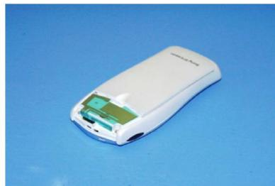
Fig. 2. A small handset with an internal multiband PIFA in 2000.
