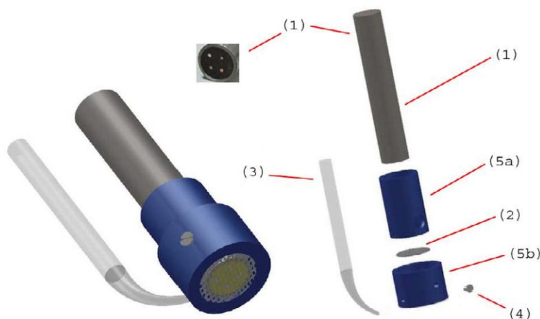
Fig. 1. Wet E-Nose sketch: (1) Electronic Nose; (2) membrane; (3) reference electrode and LPDE adapter; (4) nylon screw; (5) PVC adapters
