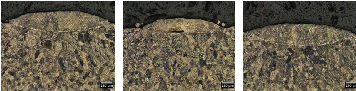
Figure 4. Metallographic picture of the cross sections of the single track samples: (a) 1; (b) 2; (c) 3.
