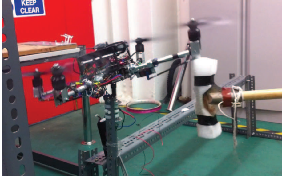
Figure 6.5: Perturbations in Roll at ball joint rig
