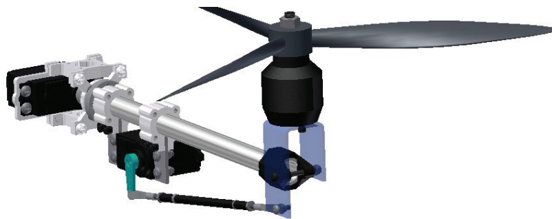
Figure 3.4: Tilting arm mechanism components
