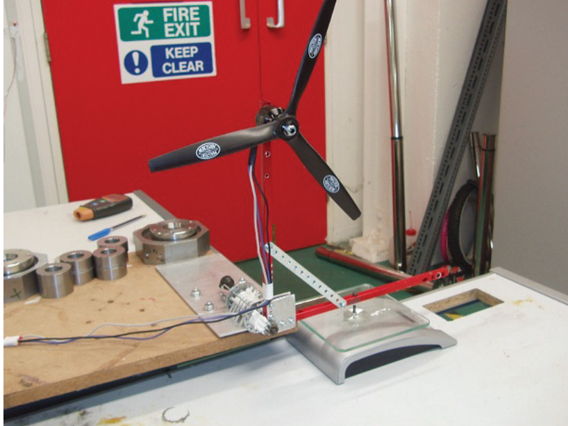
Figure 4.5: Torque Measurement Stand .
