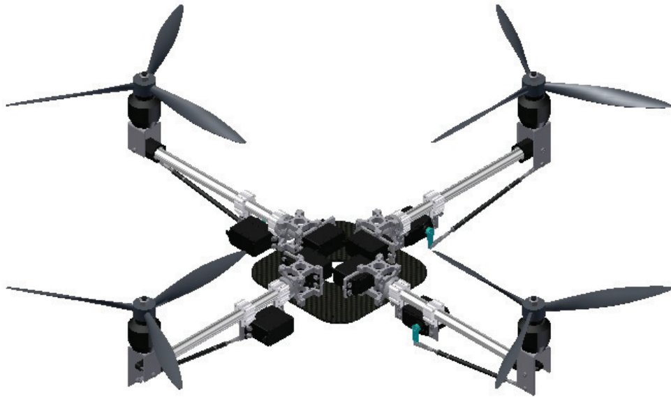
Figure 3.21: Servo blocks in the central body
