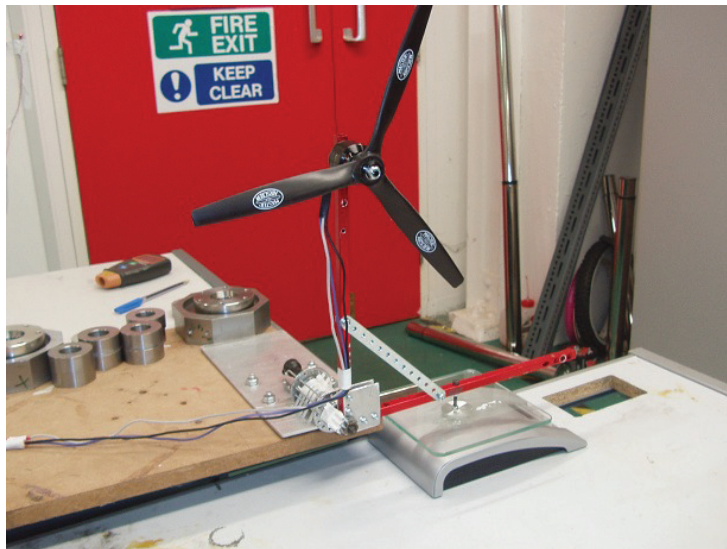
Figure A.5: Motor torque static test setup
