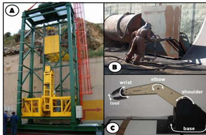
Figure 4: Tele-Operated Robots: A) EFTCoR Primary Positioning System (arm joint and joint of tracks), B) manual cleaning by an operator, C) The TeachMover Robot
