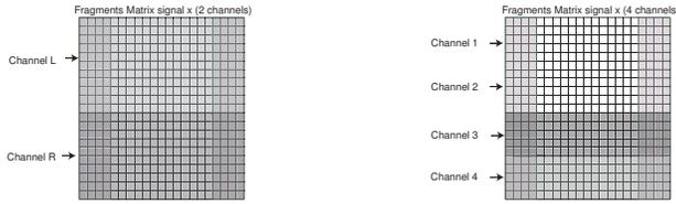
Fig. 8: The signal matrix on the left shows 2-channel resource sharing, whereas the signal matrix on the right shows 4-channel resource sharing
