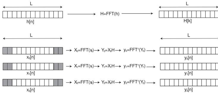
Fig. 4: Convolution of each fragment is calculated following the convolution theorem [6].
