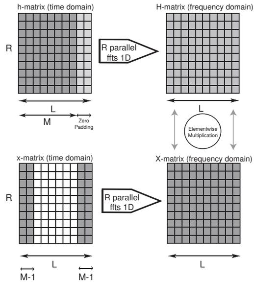
Fig. 7: FFT function from CUFFT library is applied to signal matrix and  $h$ -matrix, then an elementwise multiplication is done between them.
