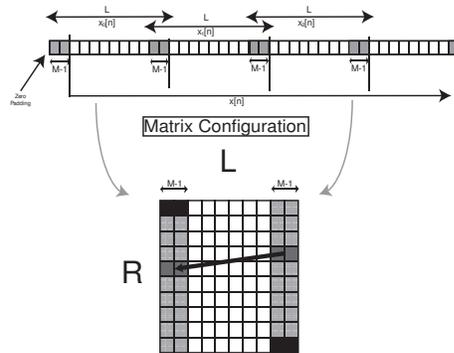
Fig. 6: A signal matrix is built from signal parts.
