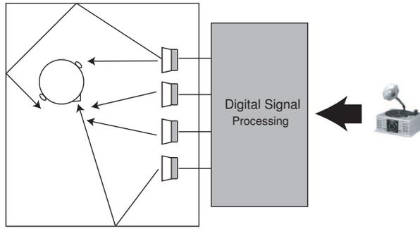
Fig. 2: Different filters applied to a sound source for audio reproduction through loudspeakers in a room
