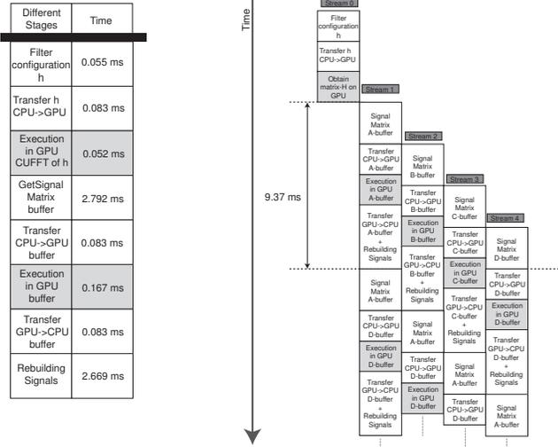
Fig. 9: Pipeline algorithm using different *streams* provided by the *concurrent copy and execution* property of GPU. On the left side, times spent by all stages of the algorithm
