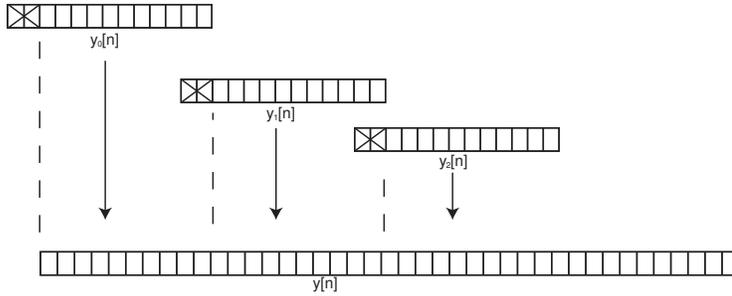
Fig. 5: As long as convolved fragments are obtained, output signal  $y$  is being formed.
