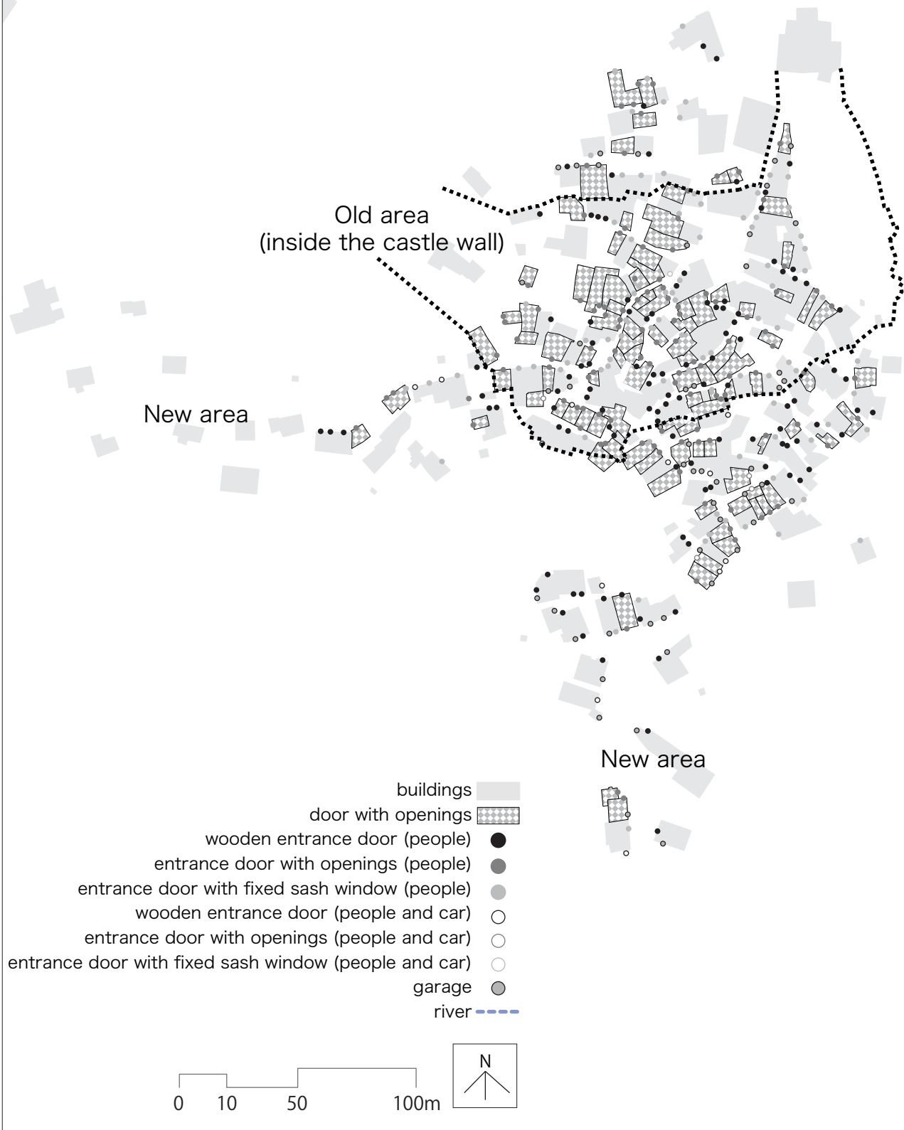
Fig.3.17 The distribution of the entrance doors in Castielfabib
