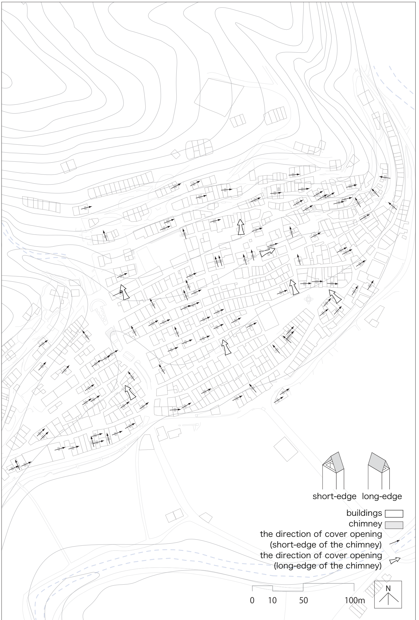
Fig.1.5 The direction of the covers of chimney in Casas Bajas
