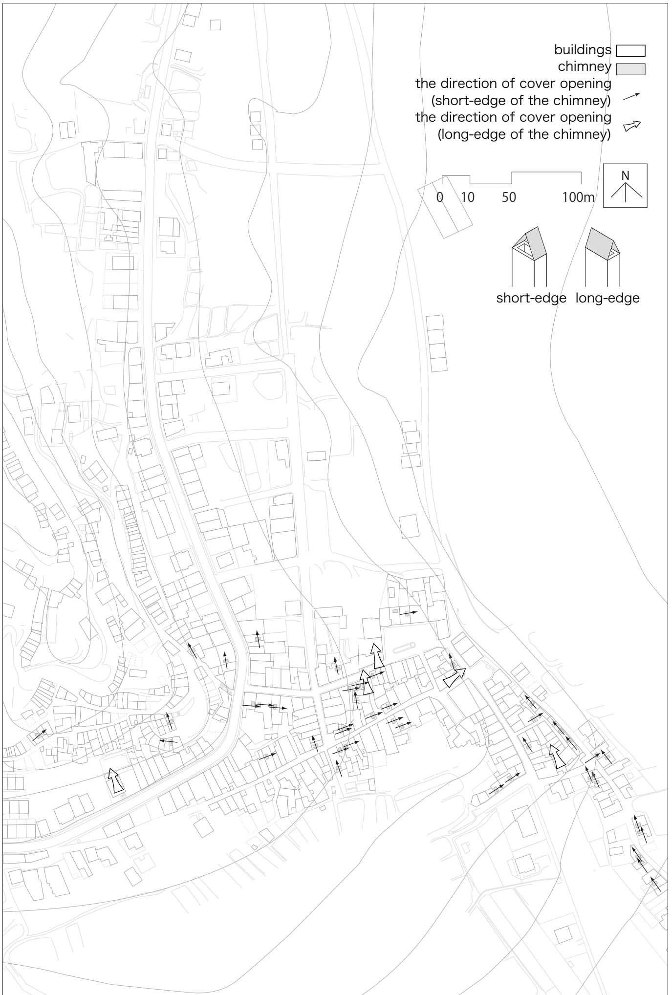
Fig.1.4 The direction of the covers of chimney in Torre Baja
