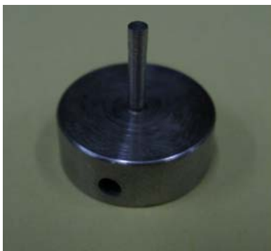
Figure 1. Machined working electrode of Alloy 926.
