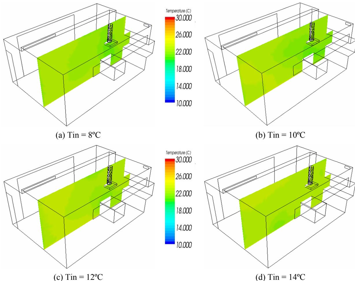
Figure 2. Air temperature in the office room
