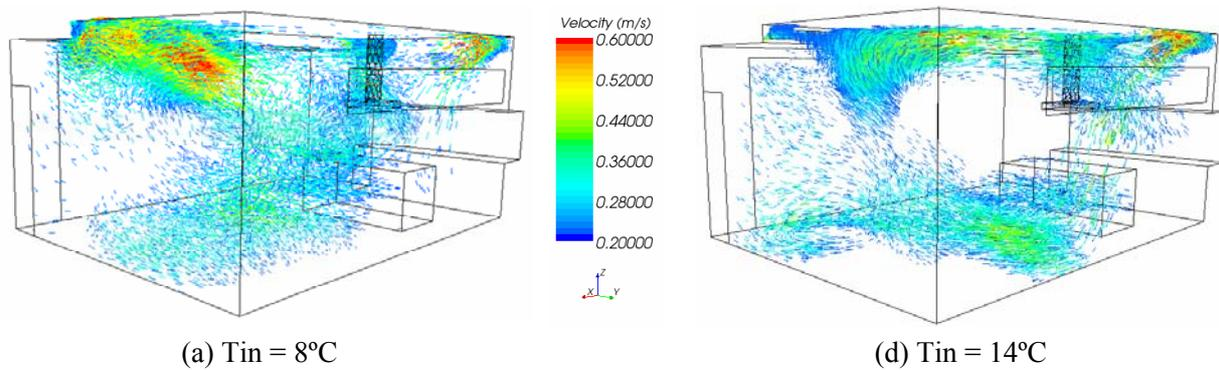
Figure 4. Air velocity vectors above 0.2 m/s (draught)
