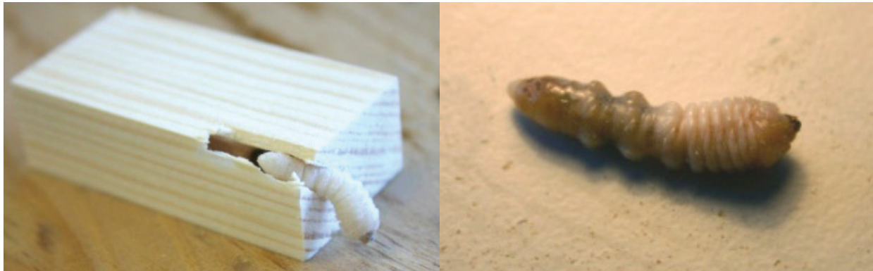
Fig. 1. Larva of a Hylotrupes bajulus before and after applying microwaves
