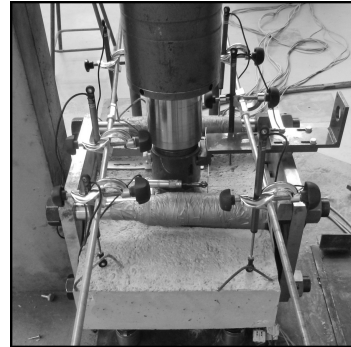
(b) Disposition of the LVDT during real test
