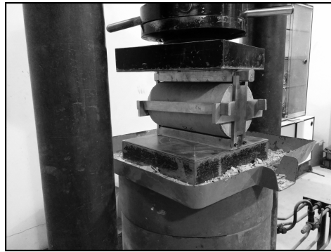
Fig. 4.5. Cylinder splitting test.
