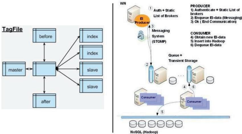
Fig. 5. Event Index Architecture: Tag Files and Data collection and Upload.
