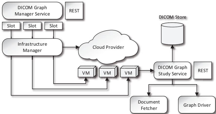
**Fig. 1.** Architecture of the graph processing framework for medical information.
