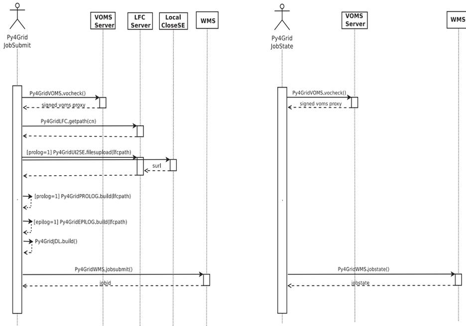
Fig. 2. JobSubmit (left) and JobState (right) sequence diagram.
