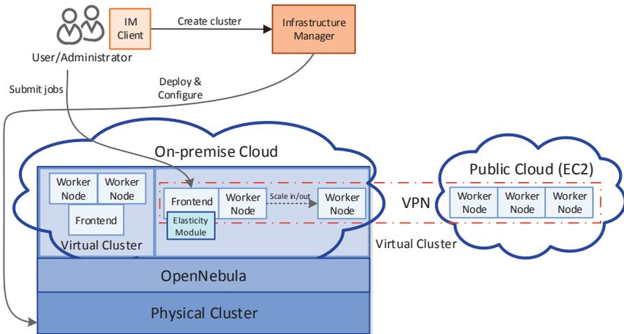
Fig. 1. Proposed cluster deployment architecture.
