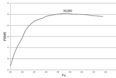
**Fig. 5.** Performance in terms of PSNR of the FPGA filter as a function of the  $F_\sigma$  parameter with  $F_t = 0.72$  in image 1.
