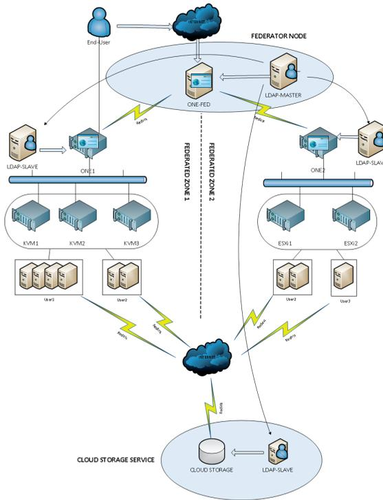
Fig. 2. Lower layer technical design. Main Items Source. FCSCCL, 2014.
