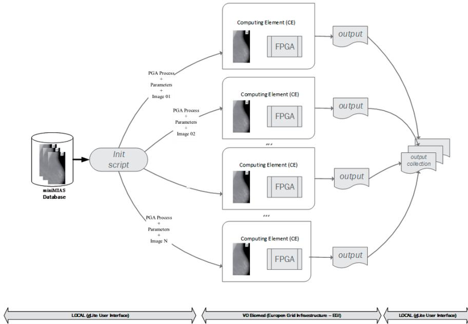
Fig. 2. Workflow of grid execution.
