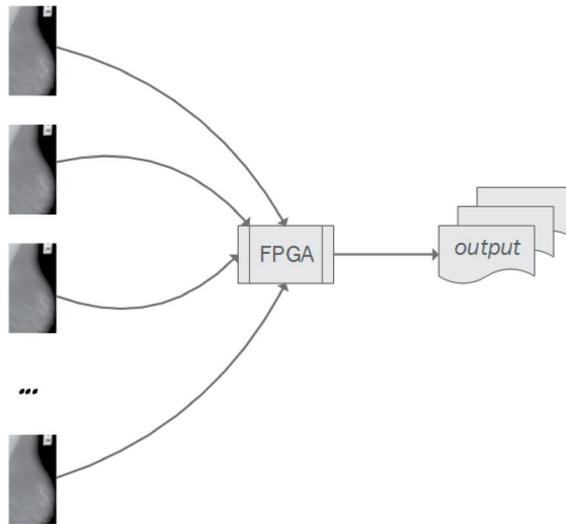
**Fig. 1.** Workflow of sequential execution.
