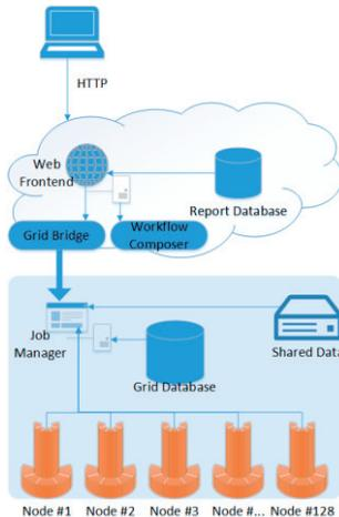
Figure 2 Component diagram for the proposed solution. Both the Grid bridge and workflow composer are deployed on the cloud for optimal accessibility and communicate with the Job manager on the login node of the Grid infrastructure.
