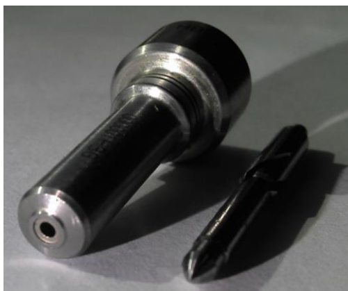
Fig. 8. Sample nozzle with the tip machined off and recessed to allow attachment of transparent tip
