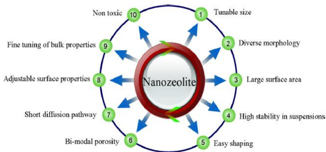
Fig 1.10 Properties of nanosized zeolites [79].
