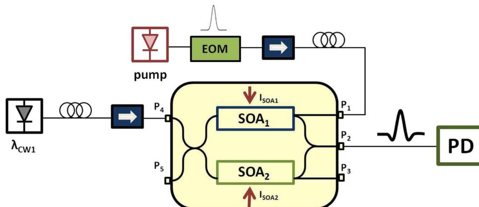
Fig. 1. Experimental setup based on a SOA-MZI.
