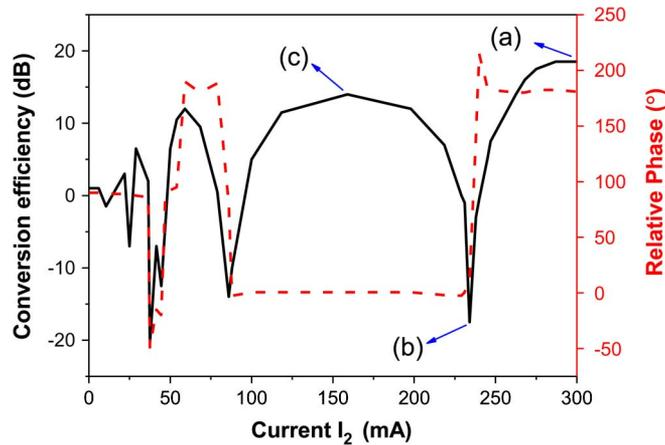
Fig. 2. Transfer function of the SOA-MZI: Conversion amplitude at the output port  $P_2$  (solid black line) and the corresponding relative phase between input port  $P_1$  and output port  $P_2$  (red dashed line). Representative operation points are labeled with letters a, b and c. Maximum conversion with a quasi-linear response corresponds with points (a) and (c) whereas minimum conversion with a quadratic response corresponds with point (b).
