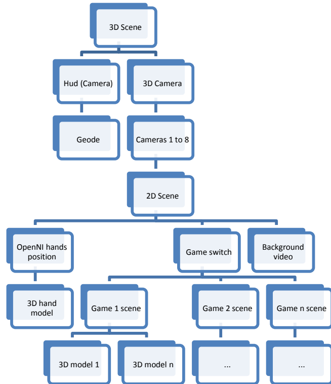
Figure 3.3: OSG graph scene used to create the 3D scene integrating OpenNI with a 3D layer specific for the autostereoscopic display
