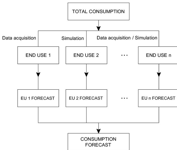
Figure 2. Consumption prediction methodology based on EUs of a building.
