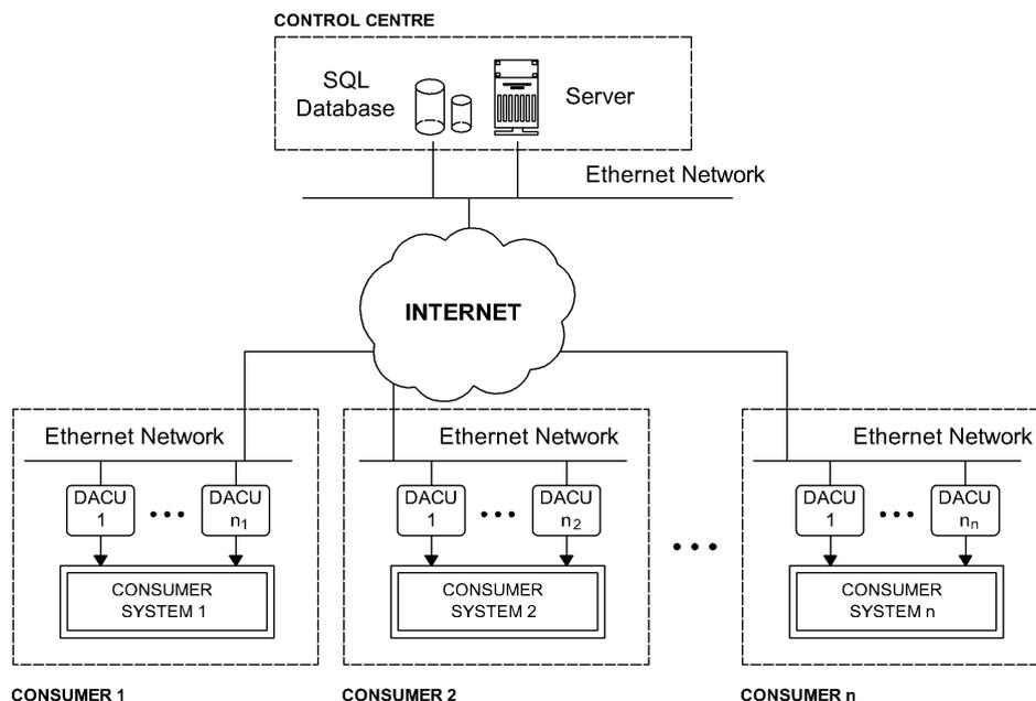
Figure 4. Recommended data acquisition architecture.
