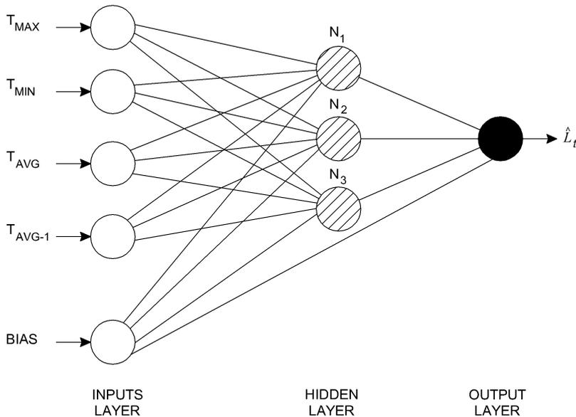
Figure1. ANN architecture used in the proposed method.
