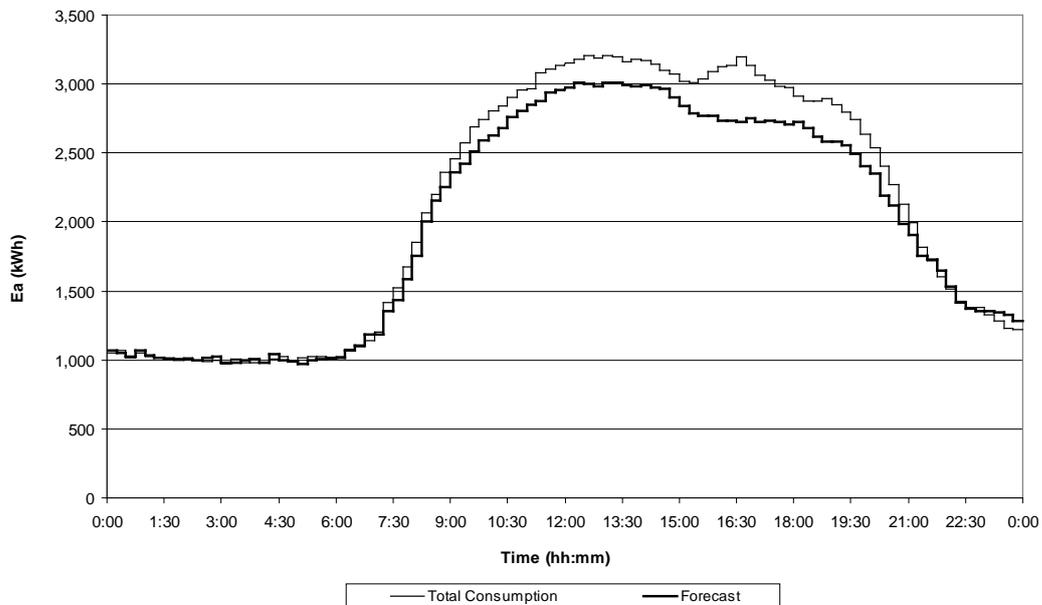
Figure 5. UPV consumption forecast for 25/06/2007 using TC method.
