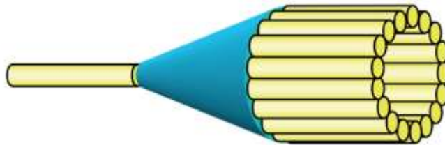
Figure 27 - Principle of the coupler with mixing elements in a conical form
