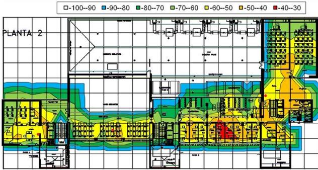
Figure 11. Radio coverage map of the second floor for UPVNET
