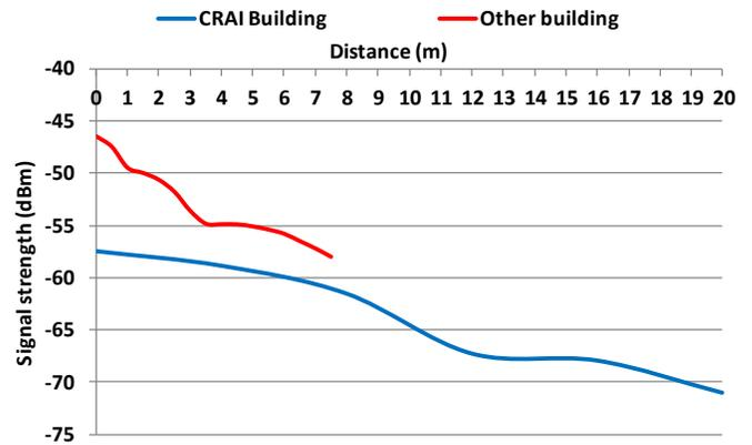
Figure 37. Signal strength for the IEEE 802.11g
