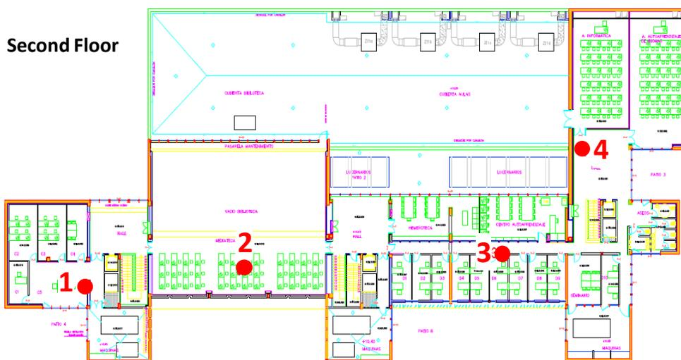
Figure 24. Relocation of APs on the second floor
