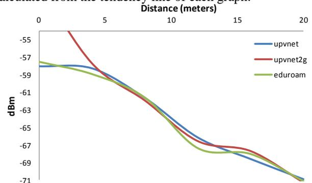
Figure 14. Signal strength on the first floor.
