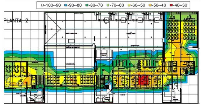
Figure 12. Radio coverage map of the second floor for UPVNET2G
