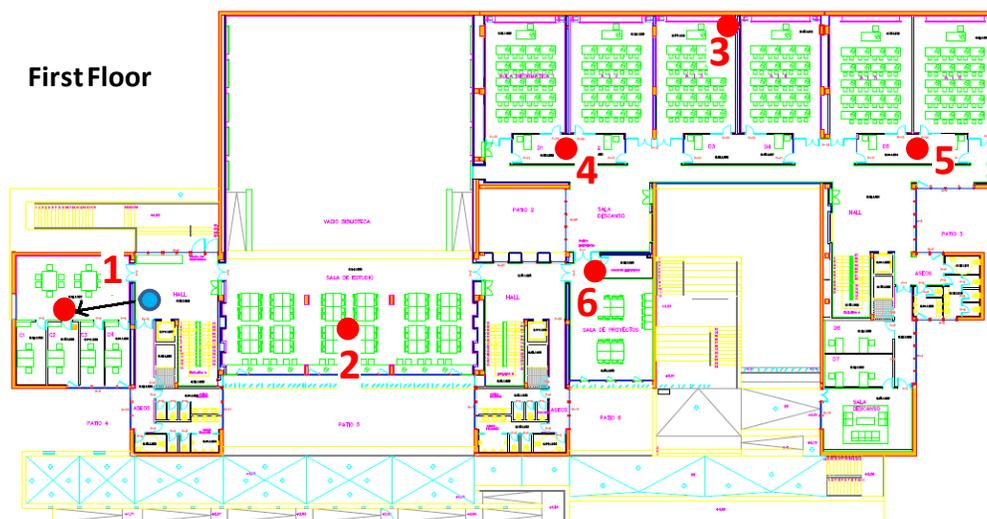
Figure 22. Relocation of APs on the first floor
