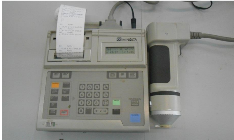
Figure 2.12. Minolta CR-300 chromameter used for determine fruit colour a , b and l .
