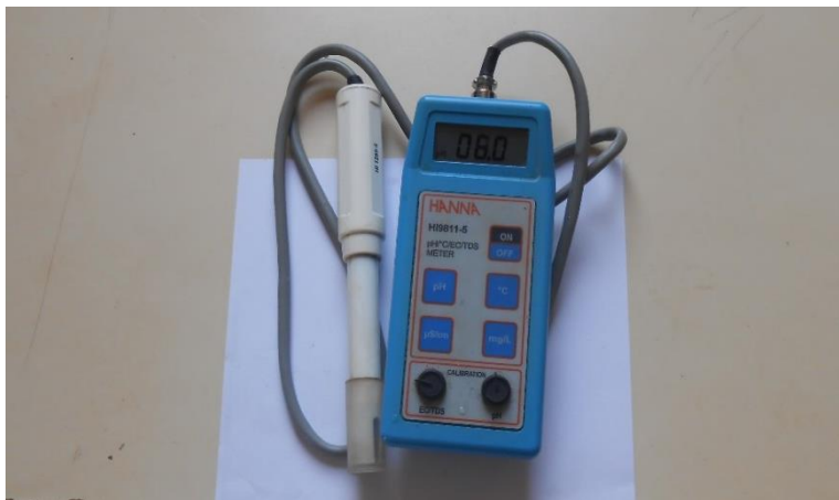
Figure 2.6. The pH/EC Meter used for measure pH and EC of the drainage water.
