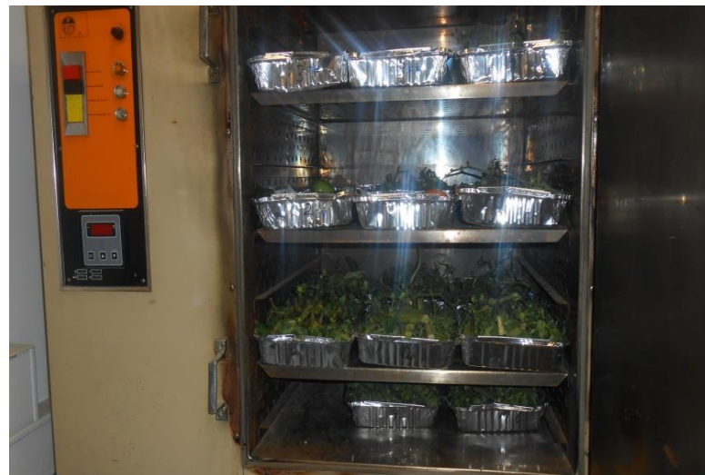
Figure 2.8. Drying of stems, leaves, green fruits and ripe/ripening fruits in the oven at 65 °C for 72 h.
