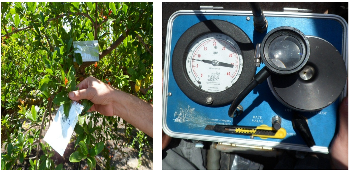
Figure 20. Stem water potential measurement, leaves covered with silver plastic bags (left) and pressure chamber used for measurement.
