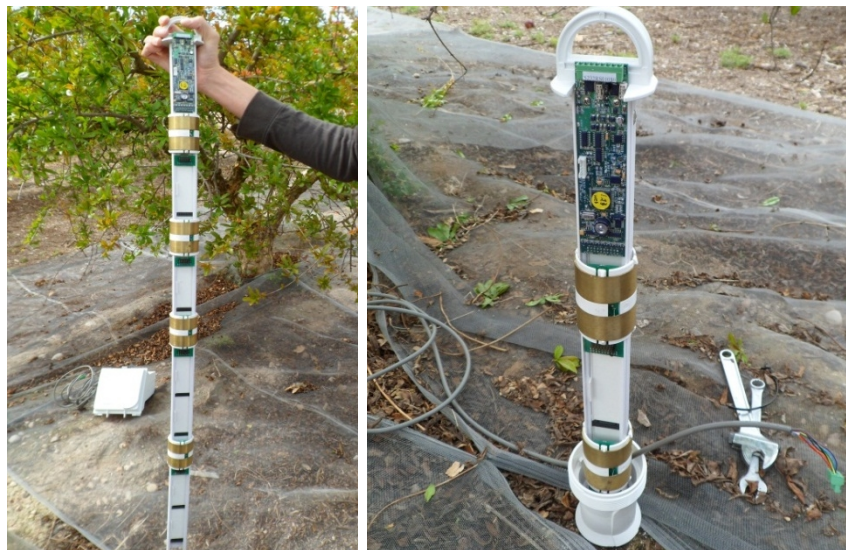
Figure 15. Installation of soil sensors.
