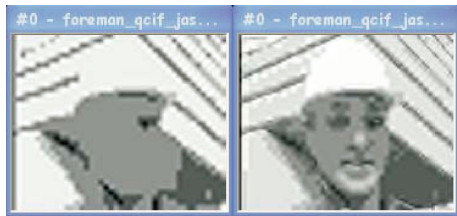
FIGURE 7: First frame of Foreman QCIF encoded at 70 Kbps (left) and 135 Kbps (right).
