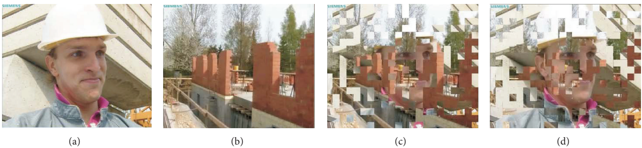
FIGURE 11: Frame reconstruction after a large burst: (a) original frame, (b) last frozen frame, and (c) (d) first and second reconstructed frames after the burst.
